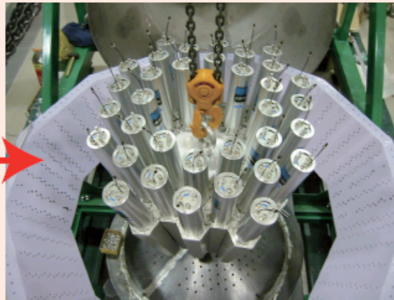
Rear panels of CsI crystals are connected with each other
