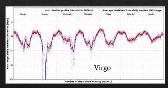
Diurnal variation of seismic noise causes diurnal variations of the detection range: demonstration of the continuous impact of the environment on detector performance
