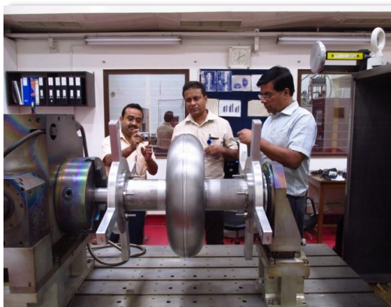
IIFC LB650 Niobium cavity, made at VECC, eb-welding at IUAC, 2K tested at Fermilab
