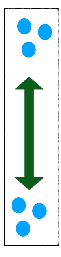
Drop a cold cloud of atoms at the top and bottom of a ~ km long vertical mine shaft
