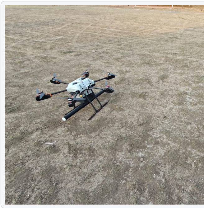
Hexacopter UAS with QuBeats sensor payload and boom-mounted vector magnetometers
