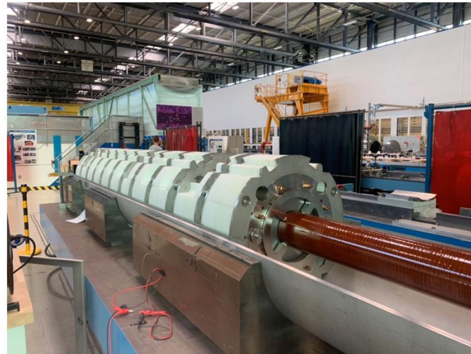
Higher Order Corrector Magnets from LASA in Italy
