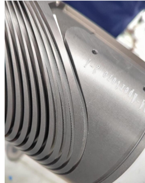
Canted Cosine Theta Corrector production at BAMA in China
