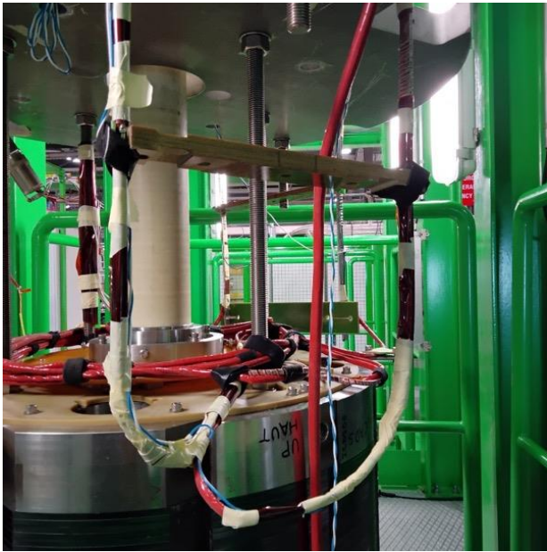
Nested dipole orbit correctors from Elytt in Spain
