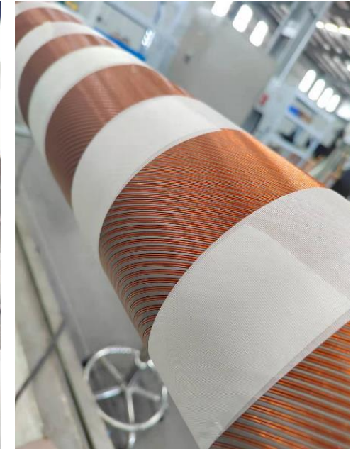
Canted Cosine Theta Corrector production at BAMA in China
