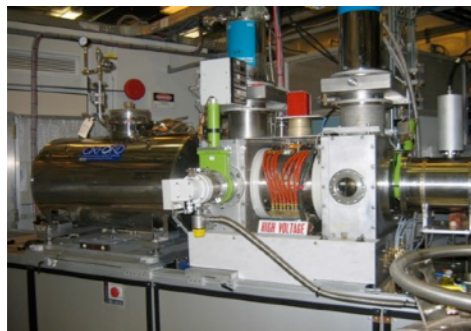
Polarized H^- ion source P = 80-85\% (at 200 MeV)
