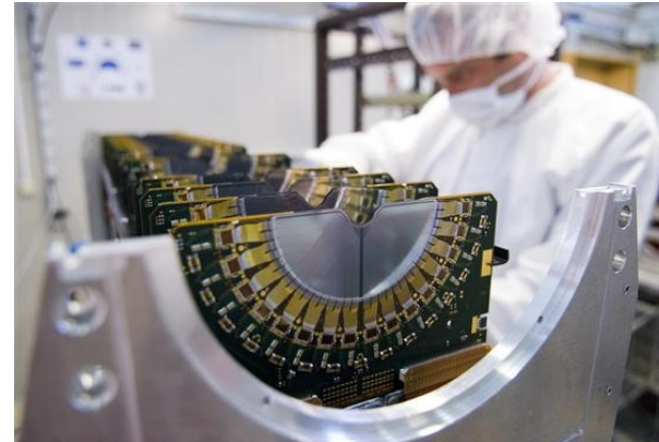
One-half of the VELO under construction
