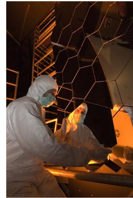
Assembling RICH 2; note the mirrors
