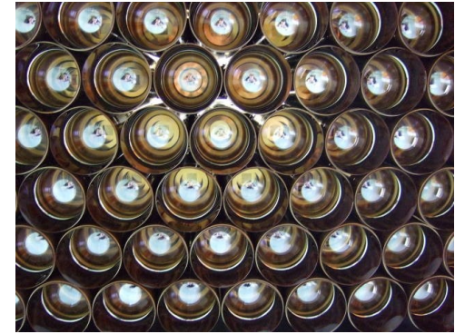
Array of RICH photodetectors
