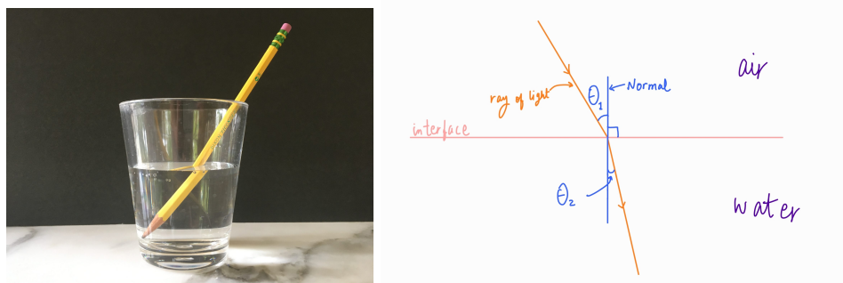
Figure 1: Left: How interesting that refraction makes the pencil appear broken! Right: This figure is the schematic showing how light bends while entering a denser medium. \theta_1 and \theta_2 are the angles between the ray of light and the normal at the air-water interface.
