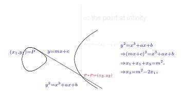
■ The double of the point P = (x, y) is given by  $2P = P \oplus P = (x_3, -y_3)$ .
