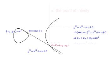
■ The double of the point P = (x, y) is given by  $2P = P \oplus P = (x_2, -y_2)$ .
