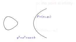
■ The point ① serves as the identity for addition on elliptic curve.
