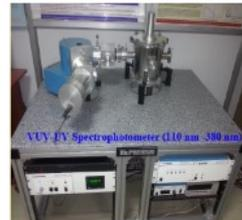
VUV-UV Spectrophotometer (110 nm - 580 nm)
