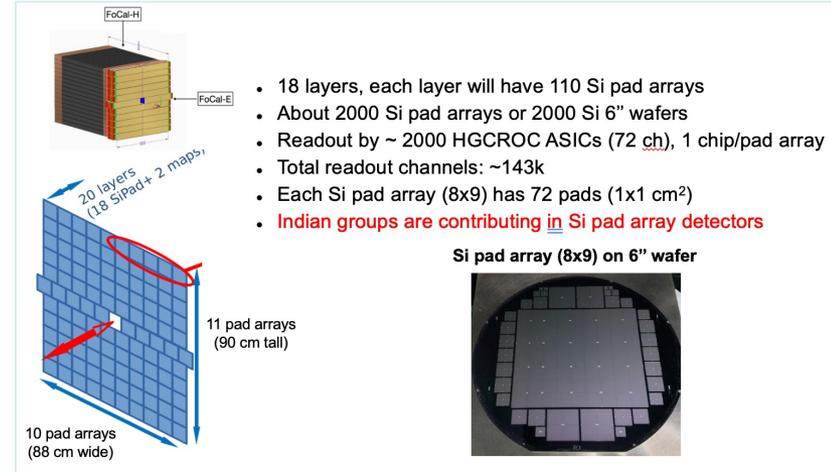
ALICE Forward Calorimeter (FoCal): FoCal-E and FoCal-H
