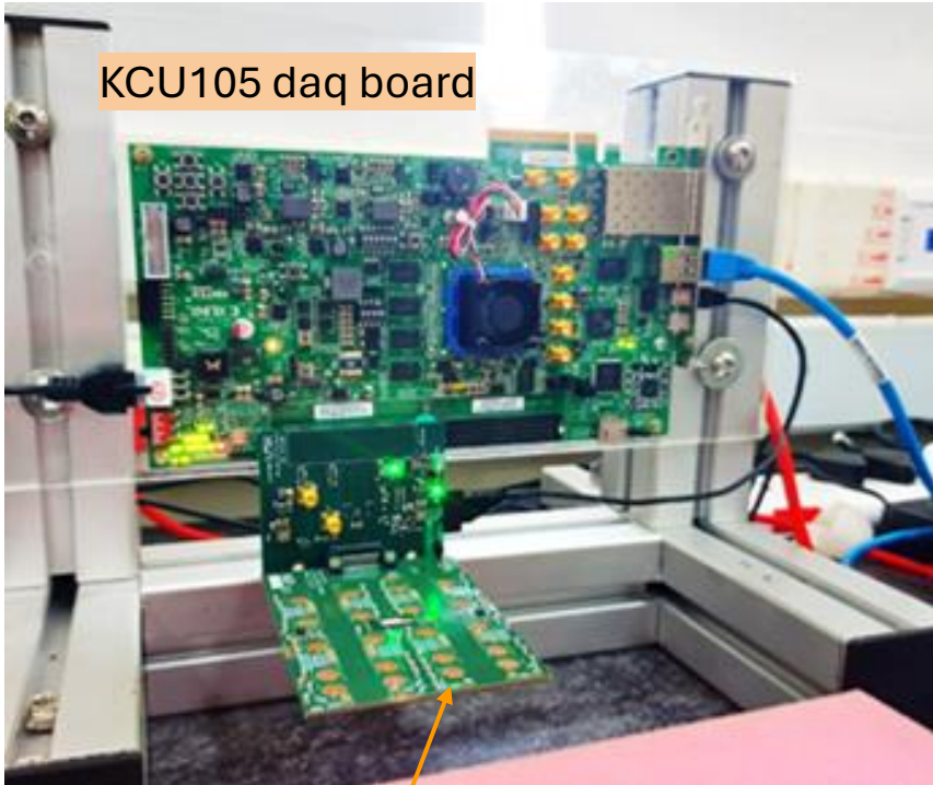
Detector connected with HGCROCV2 PCB
