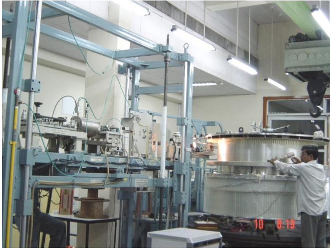
Superconducting Magnet coil winding facility, VECC
