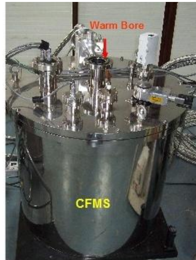
Cryofree High T_c Superconducting Magnet, 6.2 T, IUAC
