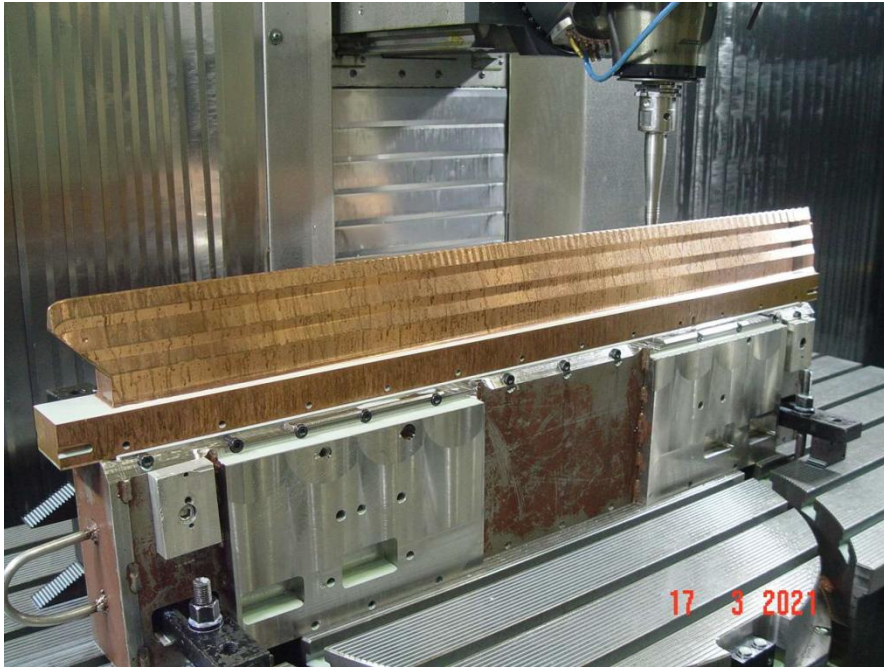
Development of 3Mev Radio Frequency Quadrupole, RRCAT
