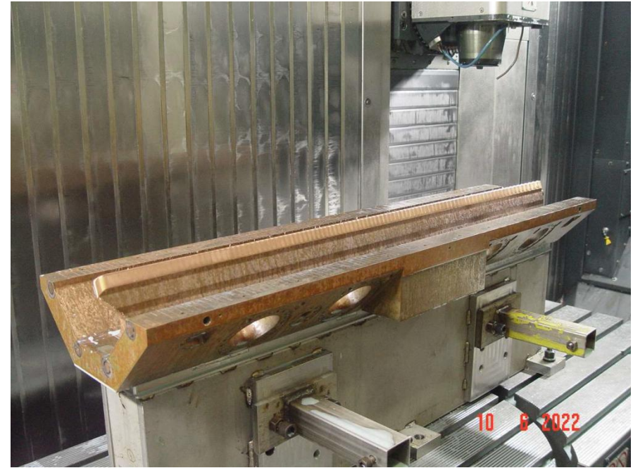
Development of 3Mev Radio Frequency Quadrupole, RRCAT
