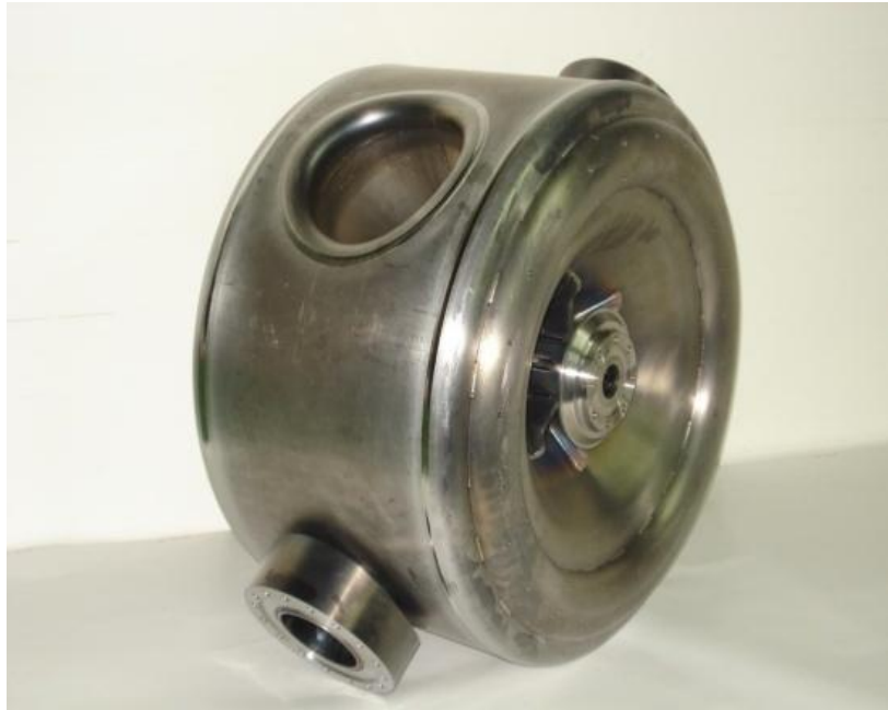
Spoke Cavity, 352 MHz, \beta = .22 IUAC-BARC
