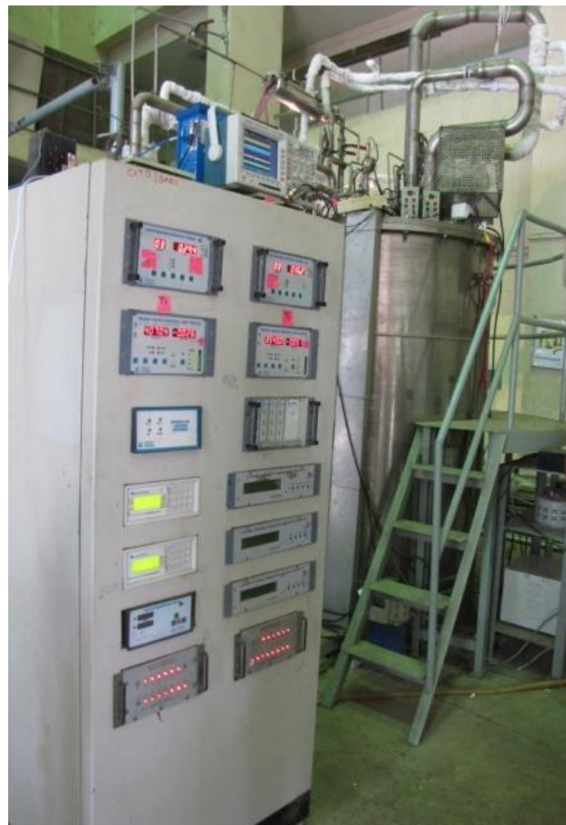
20K Helium Refrigerator Developed at BARC
