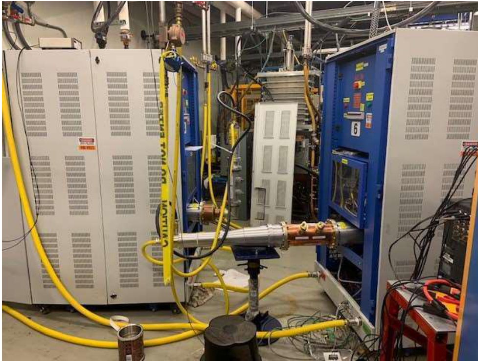
32 kW/ 650 MHz RF amplifier testing at FNAL and results up to 32 kW
