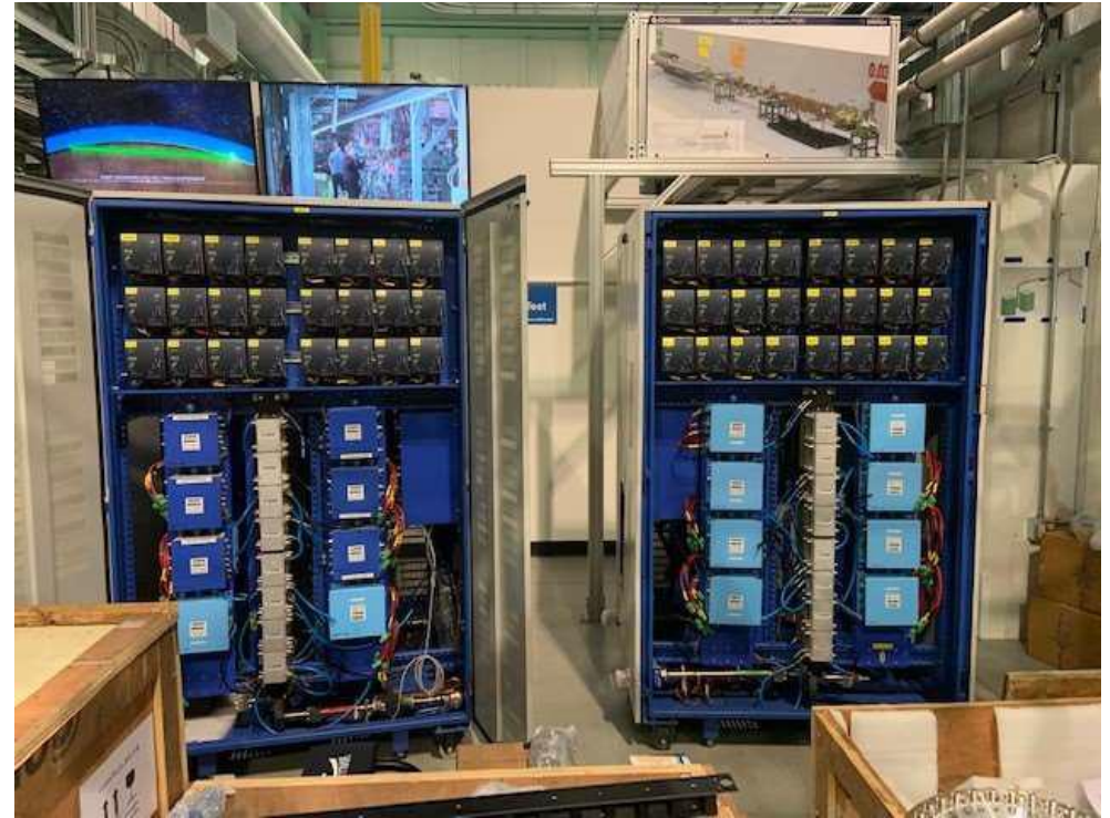
40 kW/ 650 MHz RF amplifier testing at FNAL and results up to 40 kW
