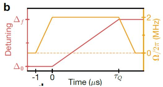
Ramping across phase transition and measuring density of defects in antiferromagnet.
