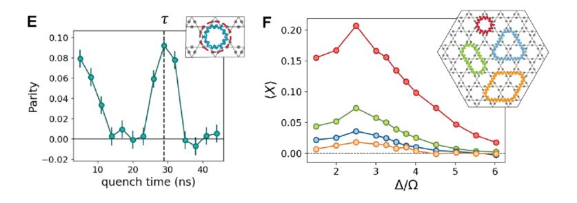
X parameter (coherence) measured by quenching and measuring Z parity
