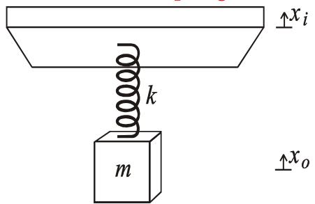
The input is the position of the top of the spring, and the output is the position of the mass.
