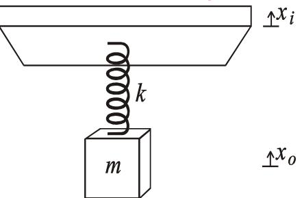
The input is the position of the top of the spring, and the output is the position of the mass.
