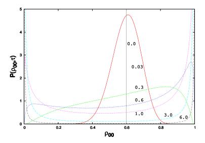
Distribution of the quantum measurement trajectories for quantum diffusion evolution of a qubit. The initial state is  $\rho_{00}(\tau=0)=0.6$ , and the curves are labeled by the values of the evolution parameter  $\tau\equiv\int_0^tg(t')dt'$ . The narrow initial distribution splits into two non-interfering components that converge to the measurement eigenstates at  $\rho_{00}=1,0$  as  $\tau\to\infty$
