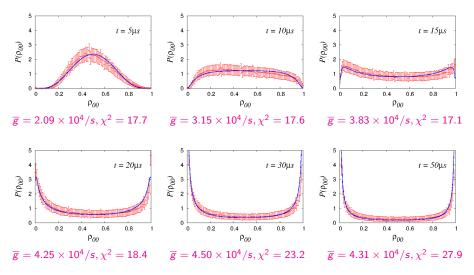
Evolution of the quantum trajectory distribution for weak Z-measurement of a superconducting transmon qubit initially polarised along the X-axis. The histograms represent the experimental data for an ensemble of  $4\times10^5$  trajectories. The curves are the fits to the quantum diffusion distribution, with a single evolution parameter  $\tau=\overline{g}t\in[0,2.2]$ .
