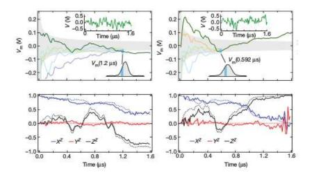
Observed quantum trajectories for weak Z-measurement of a superconducting qubit. The initial state is polarised along the X-axis. The top panels show the measured voltage distribution as a function of time, together with a few individual contributions. The lower panels display quantum trajectories obtained from the measured signal (dotted lines), and those reconstructed using tomography (solid lines).
