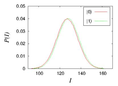
Observed probability distributions of the weak measurement signals for the two eigenstates of superconducting transmon qubit. They are approximate Gaussians, slightly displaced from each other. ( $\Delta I = 1.016 \ll \sigma = 9.99$ )
