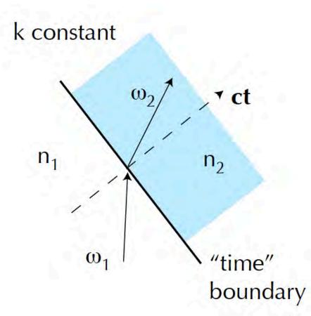
A spatially uniform, time-varying medium leads to a time-dependent frequency of any propagating waves.
