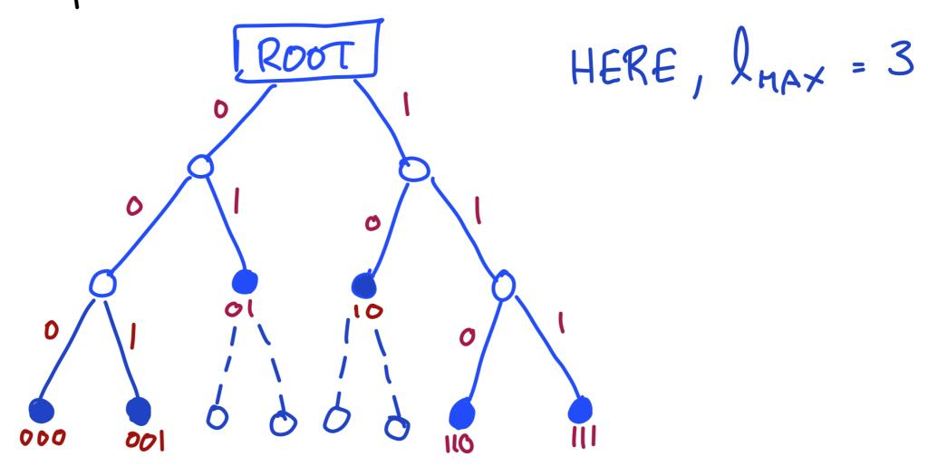
A CODEWORD AT LEVEL  $l_k$  HAS  $2^{l_{MAX}} - l_k$  DESCENDENT NODES AT LEVEL  $l_{MAX}$ . ALL THESE DESCENDENT NODES FORM DISJOINT SETS. MOREOVER, THE NUMBER OF NODES IN THESE SETS MUST BE LESS THAN OR EQUAL TO  $2^{l_{MAX}}$ .
