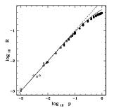
Solid line: analytical result; Dotted line:  $\mathcal{R}=p$ Points: Simulations (with different lattice sizes N=10,50,100,500) (Sinha, 2002)
