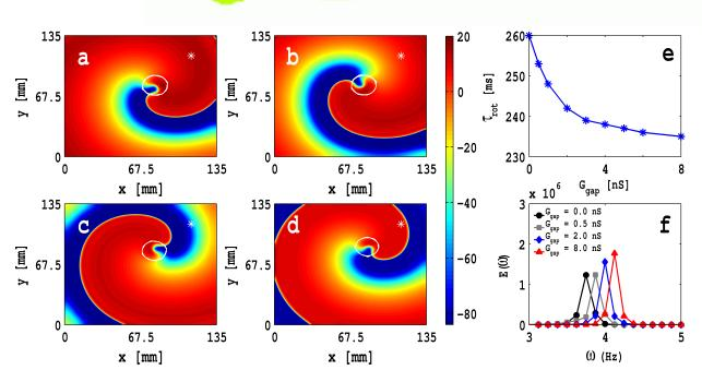
Pseudocolour plots of  $V_m$ , in a square simulation domain of side L=135 mm, at time t=2 s with  $G_f=4.0$  nS,  $E_f=-39.0$  mV, zero-sided coupling with  $D_{mm}=0.00154$  cm $^2$ /s, and (a)  $G_{gap}=0.0$  nS (control case, i.e., only myocytes), (b)  $G_{gap}=0.5$  nS (low coupling), (c)  $G_{gap}=2.0$  nS (intermediate coupling), and (d)  $G_{gap}=8.0$  nS (high coupling).
