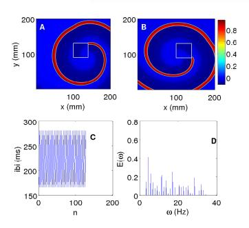
The spiral wave gets anchored to the inhomogeneity. Here  $\epsilon_1^{out}$ =0.01 and  $\epsilon_1^{in}$  = 0.02. The inhomogeneity is placed at (100 mm, 90 mm). Though the spiral gets anchored, its motion is quasiperiodic.
