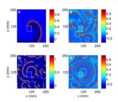
Unsuccessful to control spiral turbulence in Panfilov model with obstacle
