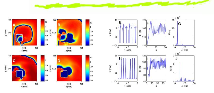
Different quasiperiodic motion observed inside and outside inhomogeneity with three underlying incommensurate frequencies in each case. Here the inhomogeneity of side l=33.75 mm is placed at (x=22.5 mm, y=22.5 mm) with  $G^{out}_{CaL}=0.000175$  (maximal value) and  $G^{in}_{CaL}=0.00003$ .
