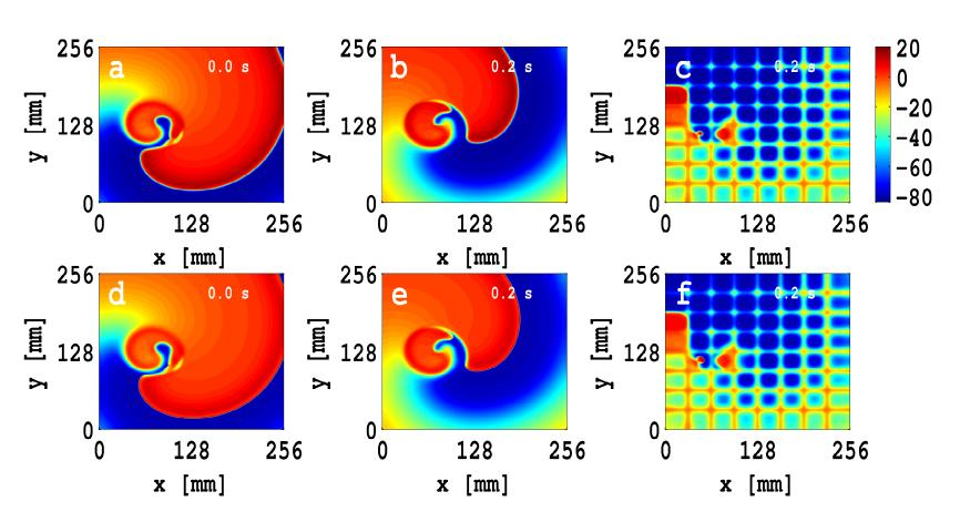
Control of spiral wave turbulence in both E and P layers by using our low-amplitude, mesh-based control scheme. **Animation**
