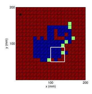
The colour of each small square indicates the final state of the system: red indicates spiral turbulence, blue a single anchored spiral, and green a quiescent state with no spirals, when the position of the lower-left hand corner of the obstacle coincides with that of the small square.
