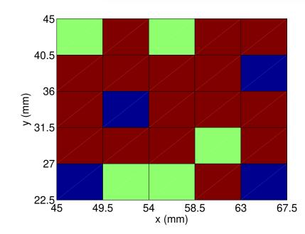
The colour of each small square indicates the final state of the system: red indicates spiral turbulence, blue a single anchored spiral, and green a quiescent state with no spirals, when the position of the lower-left hand corner of the obstacle coincides with that of the small square.
