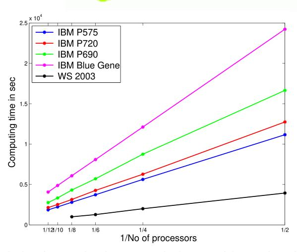
A plot of computing time versus the inverse of the number of processors for our MPI code for the TNNP model ( $600 \times 600$  domain).
