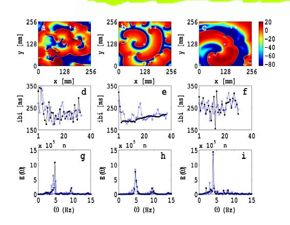
Pseudocolor plots of the transmembrane potential  $V_m$  for the TP06 model with MD along both x- and y-axes with amplitudes and frequencies (a) $A_{x,y}=0.075\ mm,\ f_{x,y}=3.0\ s^{-1}$ , (b)
