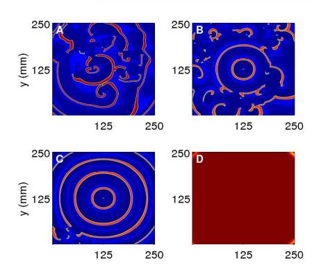
Elimination of spiral turbulence in Panfilov model by local periodic forcing, Hu et al. (2003)
