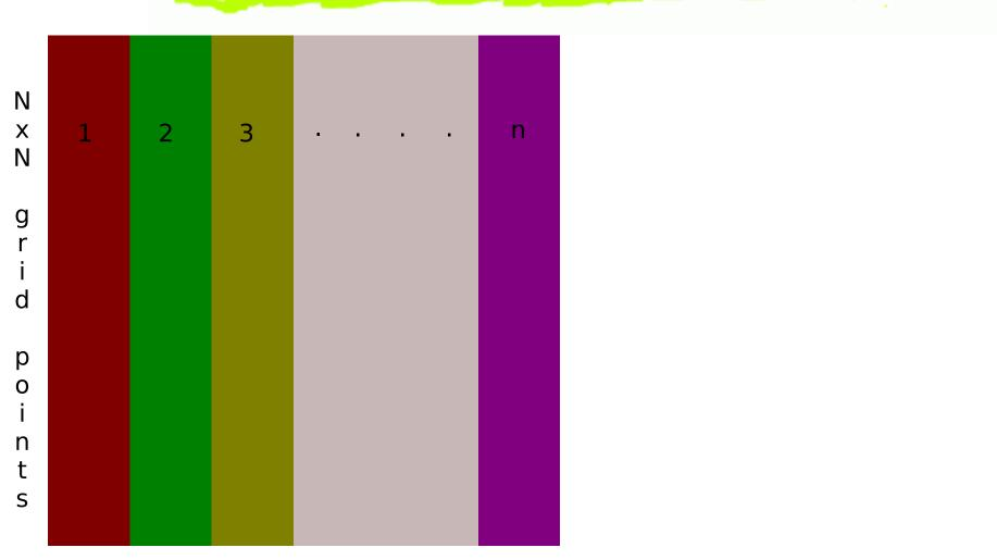
Schematic diagram of our MPI simulation, here n represents to the number of processor.
