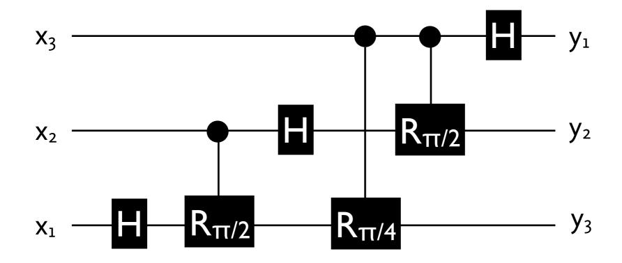
3 gates for the n=2 case; 6 gates for n=3. Scales like n2 for large n
