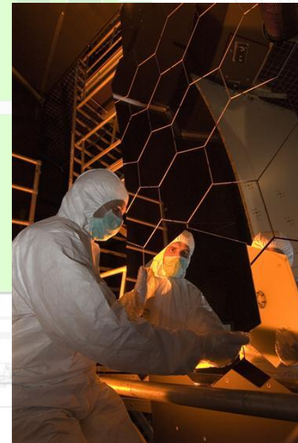
Assembling RICH 2; note the mirrors
