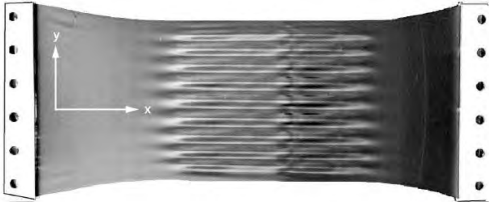
FIG. 1. Wrinkles in a polyethylene sheet of length L \approx 25 cm, width W \approx 10 cm, and thickness t \approx 0.01 cm under a uniaxial tensile strain \gamma \approx 0.10 . (Figure courtesy of K. Ravi-Chandar)
