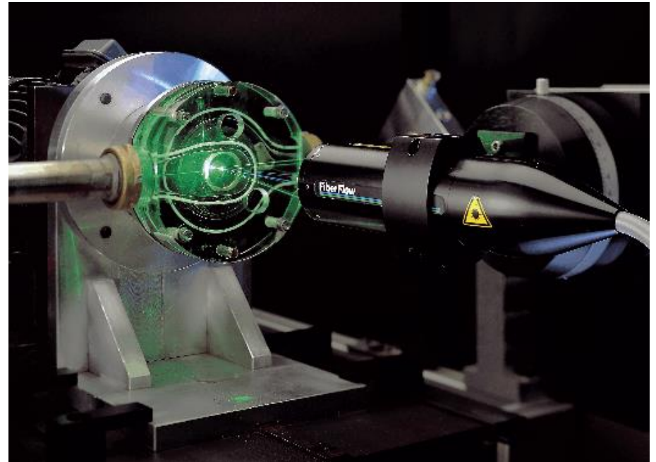
Measurement of water flow inside a pump model Photo courtesy of Grundfos A/S, DK Image from Dantec Dynamics website
