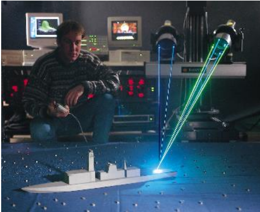
Measurement of air flow field around a ship model in a wind tunnel
