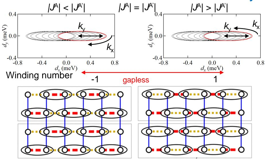
Alternation of  $J_A$ ,  $J_A$ '  $\to$  two sublattices  $\to$  nontrivial topology  $d_z(k) = 0 \to topologically protected edge states (thermally excited)$
