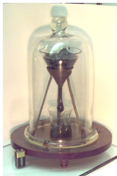
the pitch drop experiment U Queensland, Australia (1927–present) mms://drop.physics.uq.edu.au/PitchDropLive
