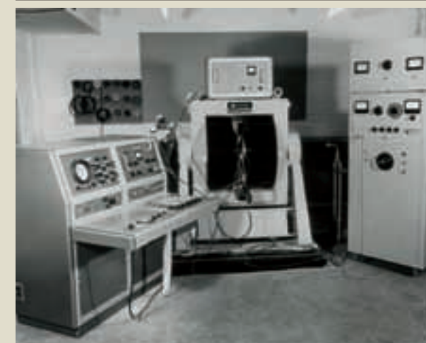
A 60 MHz high resolution NMR spectrometer used for chemical research work
