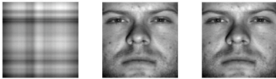
Figure 2: 1 st , 50 th , and 120 th image approximations of the image for \sigma = 0\%
