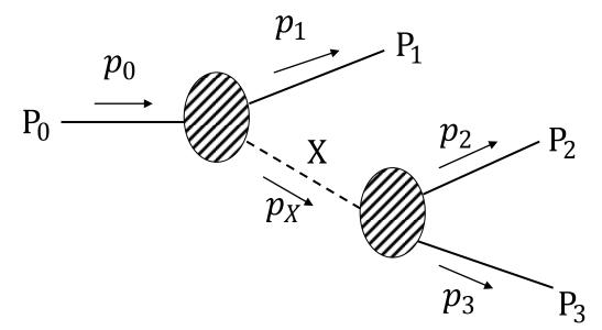
$P_0 \rightarrow P_1 + X$   $X \rightarrow P_2 + P_3$ Each is a 2-body decay X is a virtual particle i.e.  $M_X$  is variable
