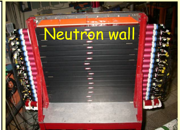
1m x 1m array of 16 plastic detectors
