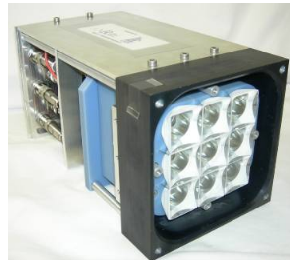
Segmented ^6\text{Li} doped glass scintillators + PMT
