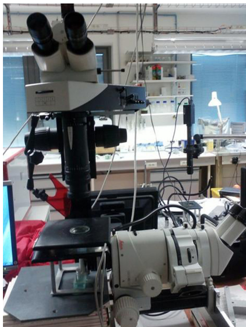
Figure 1 The experimental set-up consists of two microscopes, one conventional and the other inverted (Leica MacroFluo and Leica MZ FLIII, respectively; Leica, Wetzlar, Germany), and of two Minitüb HT300 incubators (Minitüb, Tiefenbach, Germany). The embryo is extracted from the egg and rinsed to ensure that the yolk does not blur the images.
