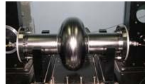
World's 1st Laser Welded Cavity
