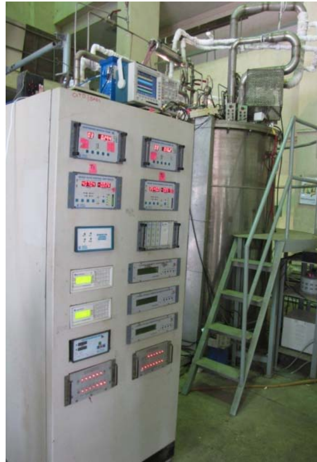
20K Helium Refrigerator Developed at BARC
