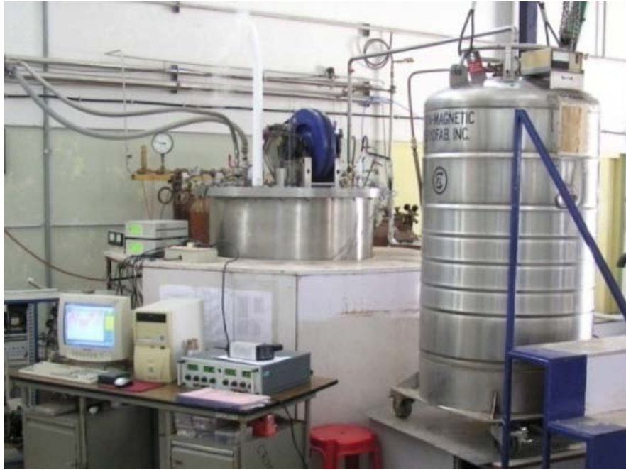
First indigenous helium liquefier, RRCAT 20-50 l/hr
