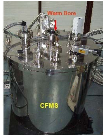
Cryofree High T_c Superconducting Magnet, 6.2 T, IUAC
