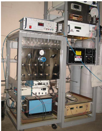
First indigenous helium liquefier, RRCAT 20-50 l/hr
