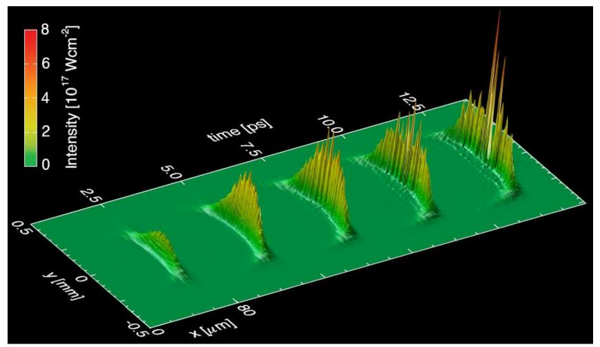
For a  $2*10^{15}$  W/cm<sup>2</sup> pump and  $\omega_0/\omega_p = 10$ , the probe is amplified, but destroyed by filamentation
