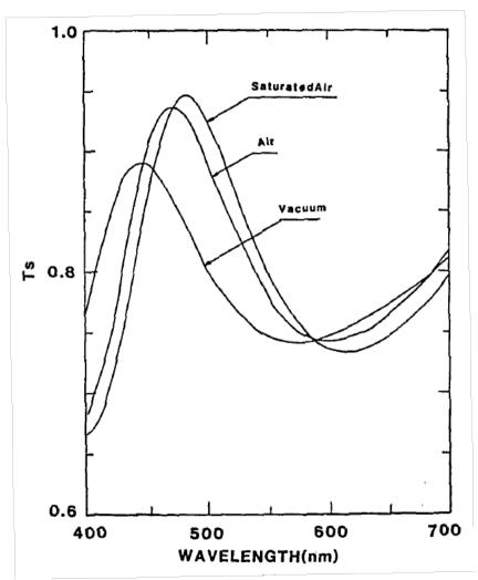
Example: transmittance vs wavelength for  $TiO_2$  films (taken from: P. J. Martin et. al., APPLIED OPTICS 22 (1), pp. 178-184 (1983) )
