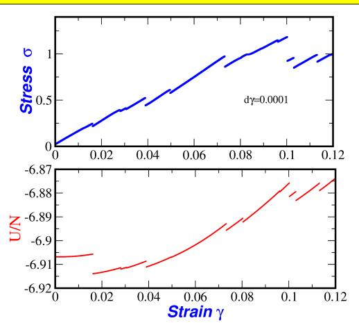
•Amorphous solids when strained, the linear elastic branches (before yielding) have plastic jumps as shown above. Local stabilty is studied by measuring the distance between two consecutive plastic drops, through Athermal Quasistatic Shear (AQS) simulations of an atomic glass former (KA binary mixture).
