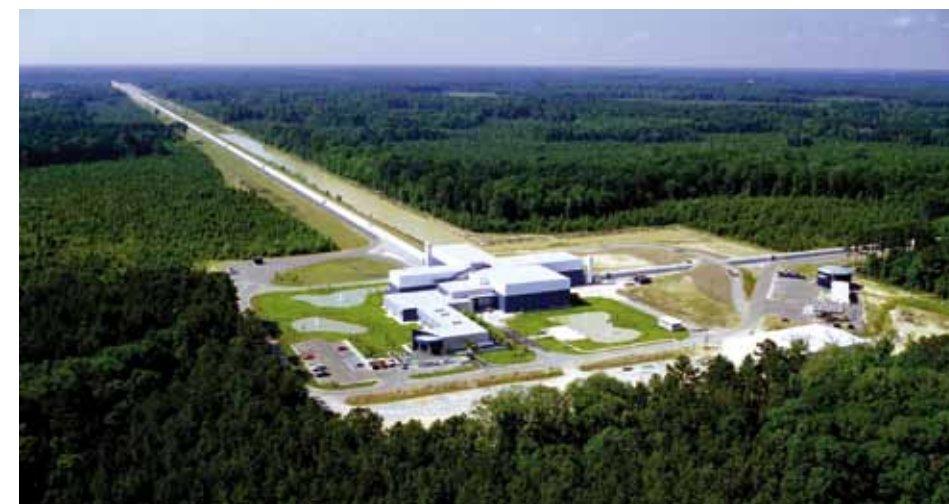
Figure 2: Aerial photograph of the LIGO-Livingston observatory in Louisiana, USA. LIGO observatories are sophisticated Michelson interferometer that have arm lengths of 4 kilometer
