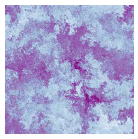
Distance traveled by fluid elements in a 3D turbulent flow during one large-eddy turnover time. Long (white) and short (purple) distances, represented here as a function of the final position in a 2D slice, define an intricate landscape with fronts where particles coming from far apart meet.
