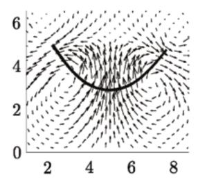
Velocity field around an unbending filament, obtained from PIV images. From Prasath et al. Phys. Rev. Fluids, 2016.
