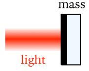
probing test-mass position perturbs momentum, causing **back-action** noise
