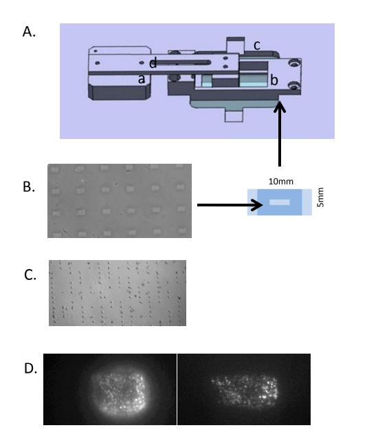
a. Linear actuator for pullingb. Mount for PDMS sheet with cells
