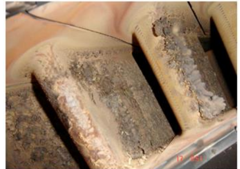
Deposition on first stage vane of gas turbine. Bons (2010)
