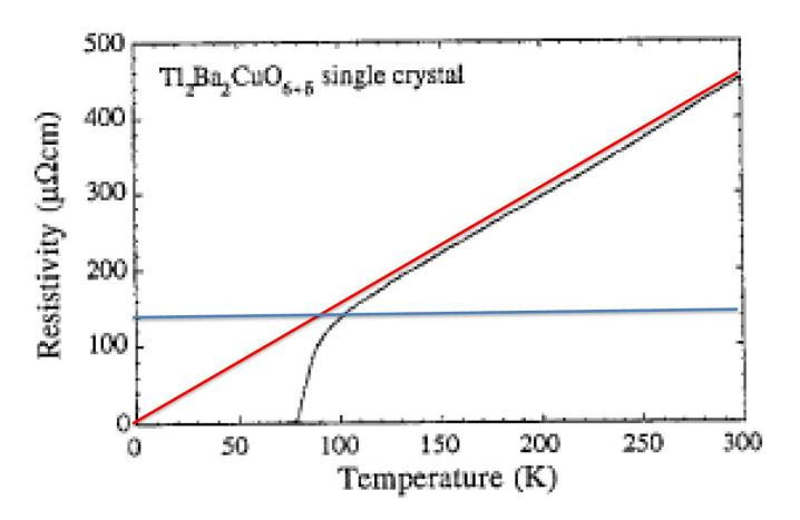
The temperature dependence of resistivity of Tl 2201 crystals for different hole concentrations can be fitted with exactly the same expression as for LSCO.
