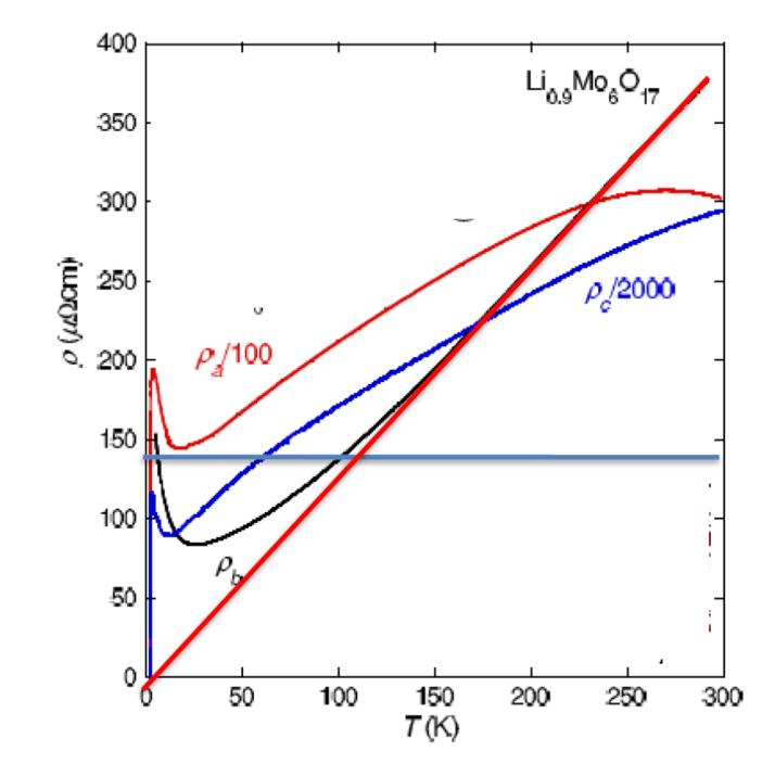
Purple bronze. Another mysterious compound. Monoclinic.Very anisotropic. Resistivity linear in T from 30 to 300K, though  $\theta_D$  ~ 400K. Metal insulator transition at ~20K. Superconductor below 2K(?).
