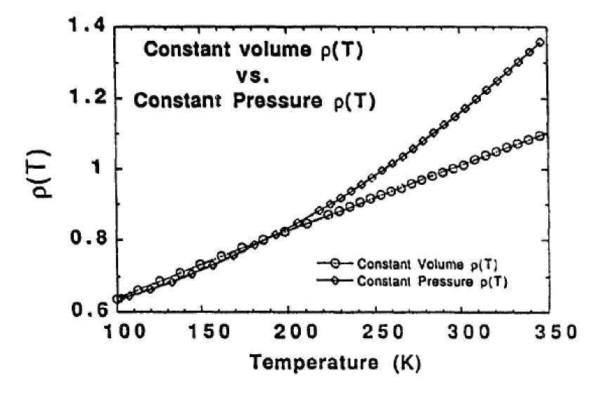
$\rho(T)$  vs.T under constant pressure (measured) and constant volume (generally calculated) for Rb<sub>3</sub>C<sub>60</sub> . (Zettl, 1994, Physica C) . The constant volume graph is really linear!
