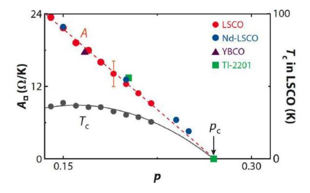
The low temperature coefficient A is common to many superconducting cuprates, as shown in the left.
