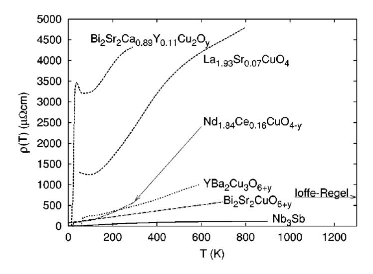
From saturation of electrical resistivity by Gunnarson, Calandra and Han, RMP 2003 Ioffe Regel limit shown for LSCO with Sr 0.07.
