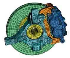
First, the solid is *discretized* into a number of elements ('meshing')
