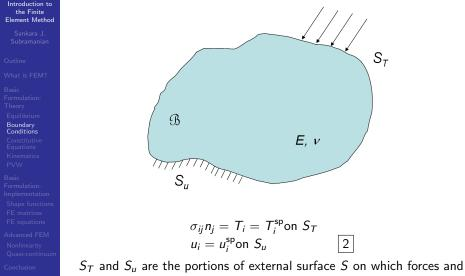
$S_T$  and  $S_u$  are the portions of external surface S on which forces and displacements are specified respectively.
